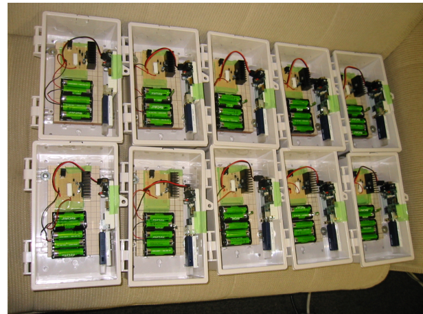
Fig. 3. DTN nodes for the experiment. People carry them by hand. They implement potential-based entropy adaptive routing.
